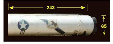
Figure 4: Minuteman III First Stage Motor
